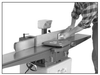
Figure 24. Typical edge jointing operation.
